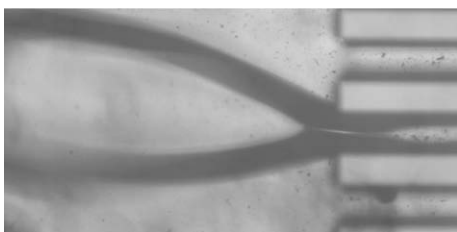
Fig. 13. Image sequence of flow boiling with HALF instabilities captured using high speed camera at frame rate of 500 fps. The vapour jet from the microchannel expands inside the inlet manifold of the heat sink.
